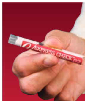
To perform test, the user first crushes the test between fingers.
