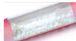
Yellow crystals lose color or change to a pale blue or green in the presence of alcohol at or above the test's threshold.
